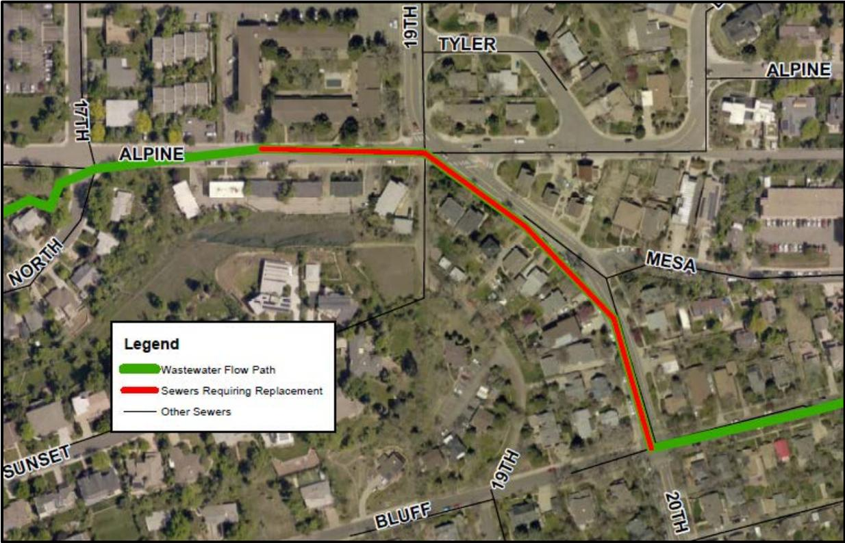
**Figure 2 - 20th St Sewers Requiring Replacement**
