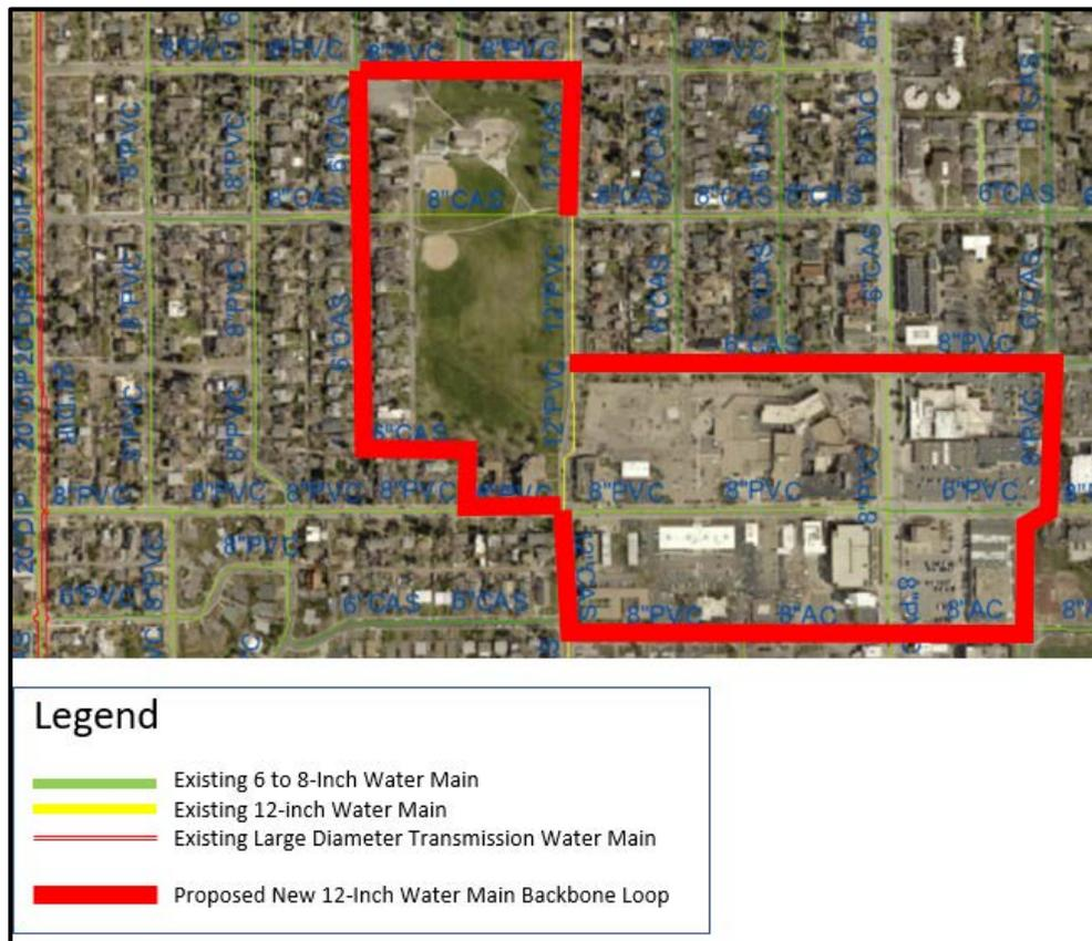
Figure 3 – Conceptual Water System Improvement
