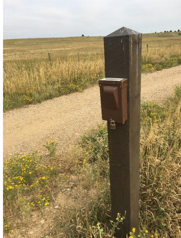
*Figure 1 Metal enclosure containing a TRAFx trail counter unit, mounted on a post along an OSMP trail/road.*
